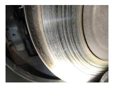
**3. BRAKES:** Front brake disc (both)
